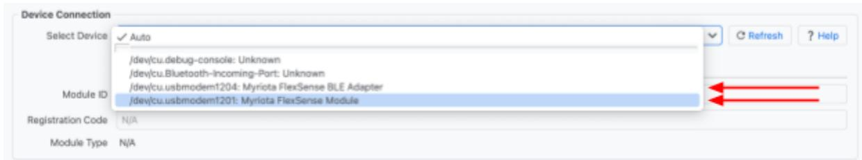
Selecting and connecting to the **Myriota FlexSense Module** enables updating the System Image, User Application and Network Information through the default screen.
