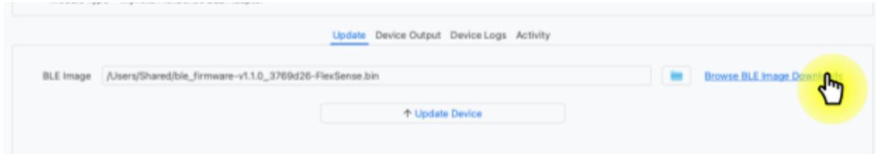
Once the file has been selected, click the **Update Device** button to program the firmware. Upon completing programming, the device may disconnect and will no longer appear as an available device in the **Select Device** dropdown. This is normal, and after the BLE completes its reboot, the device will appear as an available device when you click **Refresh**.
