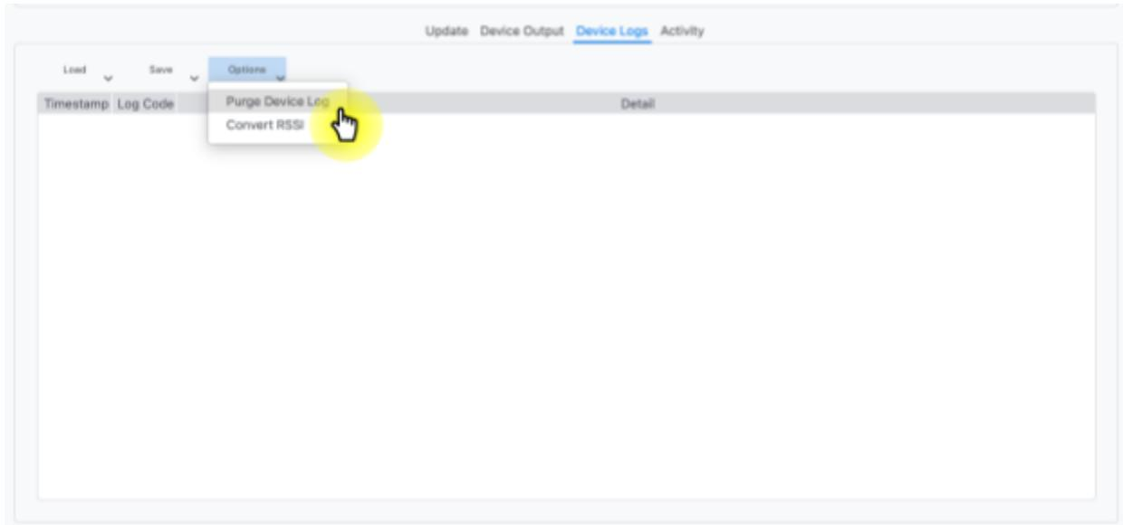
When running the RF test example in the [SDK GitHub repository](#) for non-FlexSense devices with logging enabled, the RSSI results can be converted to a human-readable format using the "**Convert RSSI**" option under the **Options** button.
